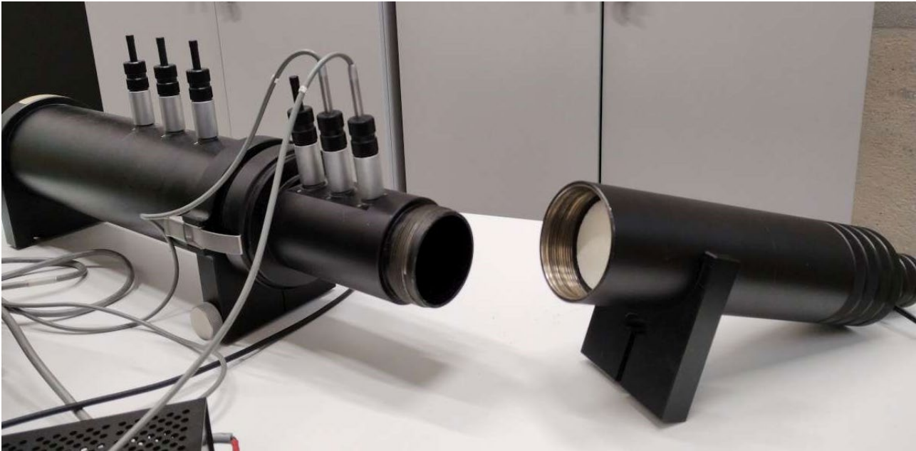
Fig. 2. An example of test piece installation in the sample tube.
